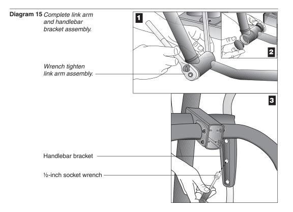
e. Wrench tighten using a <sup>9</sup>/<sub>16</sub>-inch socket and open end wrench. Refer to Diagram 15, #1.
